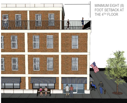
FIGURE 10: 4TH FLOOR SETBACK REQUIREMENT
