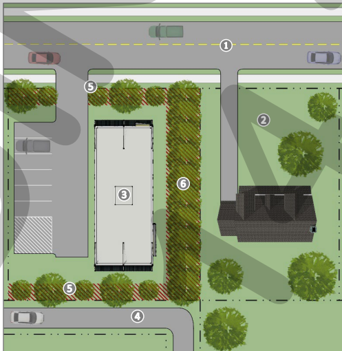
1: STREET; 2: RESIDENTIALLY ZONED OR USED PROPERTY; 3: INDUSTRIAL OR COMMERCIAL ZONING/USE; 4: ALLEYWAY; 5: TEN (10) FOOT LANDSCAPE BUFFER WITH ACCENT AND CANOPY TREES; 6: 20-FOOT LANDSCAPE BUFFER WITH THREE (3) TIERED SCREENING
